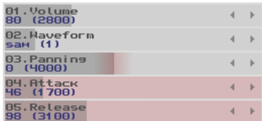
Click twice (or right click) on the controller to open the **Controller Properties** window, where you can do the following operations: change, reset, randomize, write to pattern, assign MIDI IN:
