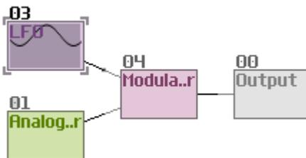
3. Generator=ON; the input is empty; output is connected to [Sound2Ctl](#); thus, the LFO can change the values of the controllers of other modules.
