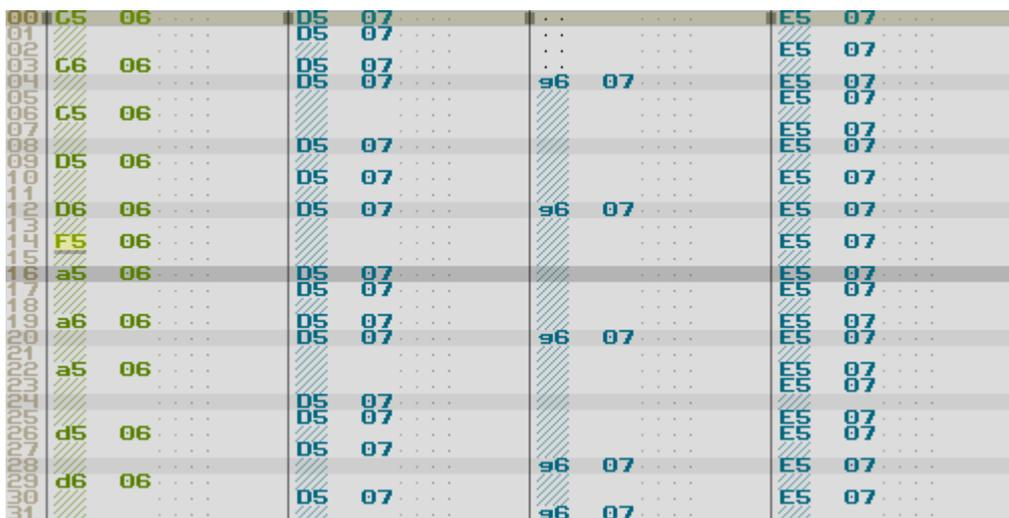
**Pattern** is a group of simultaneously played tracks that represents some section of the SunVox project (score). It is divided into horizontal lines. Playing direction is top-down.
