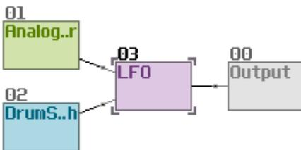
2. Generator=ON; the input is empty; at the output we get the wave of the built-in oscillator; this output signal can be used for something else, for example to modulate the volume or frequency through the [Modulator](#).
